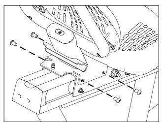
Figure 8: Attaching the seat back assembly
